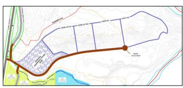
Whitehorse. The plan was prepared to provide a viable aggregate source for private industry, the City of Whitehorse, Yukon Government and Kwanlin Dün First Nation. The plan details how extraction should proceed in order to minimize impacts on adjacent land uses and includes pit operation and reclamation guidelines.
